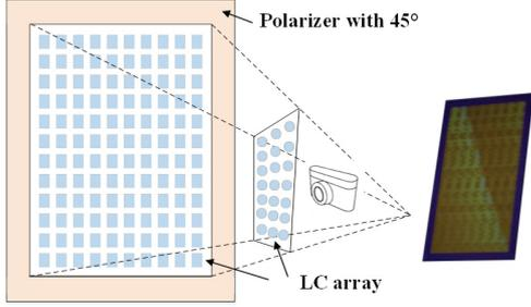
Fig. 12: Perspective distortion due to the shift of view angle. A polarizer is attached around the LC array to detect the polarized signal region.
