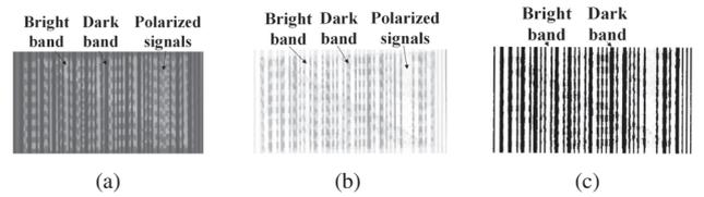
Fig. 11: Noise elimination by subtracting polarization background. (a) The noise of polarized signals in the bright band. (b) The result of noise elimination. (c) LED signal recovered by combining (a) and (b).
