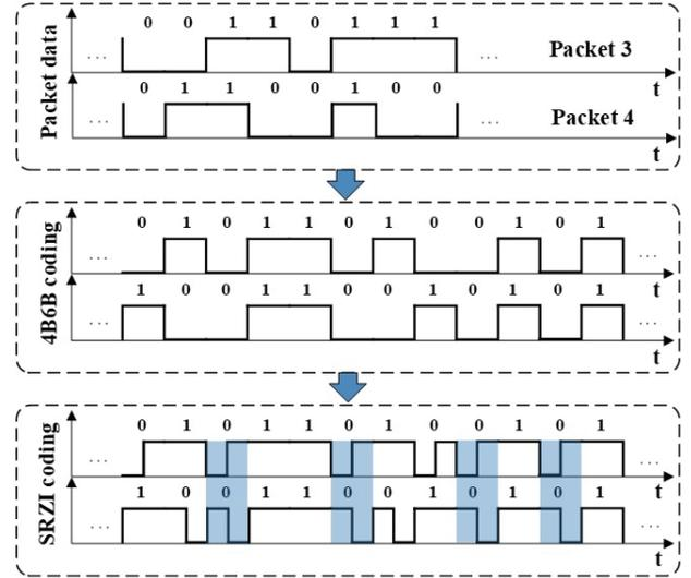
Fig. 8: Two packets are encoded with 4B6B and SRZI. These two packets first apply 4B6B for flicker mitigation, and then are encoded with SRZI for dark band elimination.
