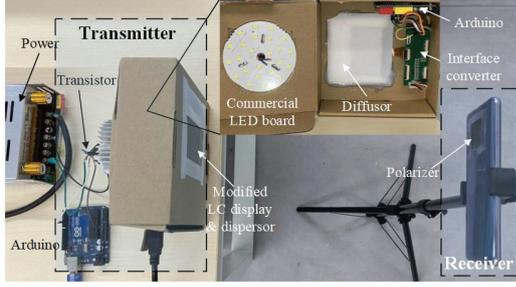
Fig. 15: Experiment setup.
