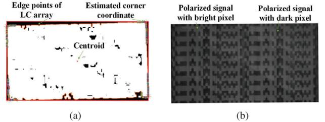
Fig. 14: The distortion image is corrected with corner coordinates. (a) Four corner coordinates are estimated by calculating the maximum distance from the centroid to edge points of LC array. (b) The final corrected image of polarized signals.
